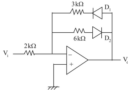
In the above circuit, assuming op-amp,  $D_1$  and  $D_2$  are ideal, if  $V_i = 2$  volts, the o/p  $V_o$  is
