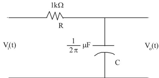
If  $V_i(t)$  is a sinusoidal signal of frequency 1 kHz, then  $V_o(t)$
